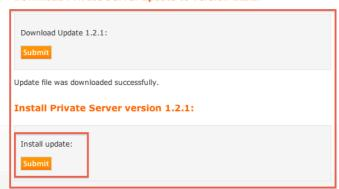
Clicking on "Submit" button under Install Update will install the downloaded patch file. The patch file will unpack and install the changes to the Virtual Appliance. The last line should say "DB successfully updated".
